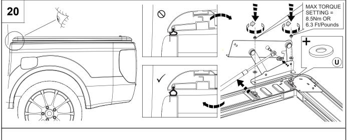
After installation carefully and thoroughly clean all debris from the inside of the cargo box. **Retain these instructions for future reference**
